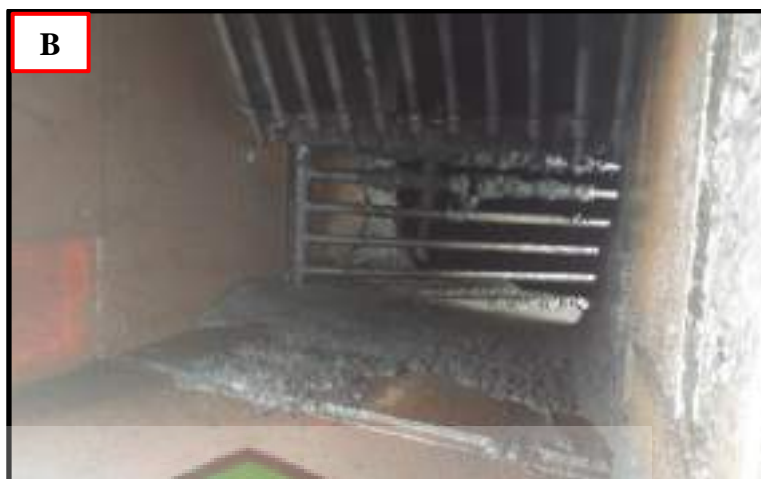
Gambar 4.6 Tempat Bercampurnya Batubara Di (A. Transfer Station ) Oleh Alat (B. Screening )
